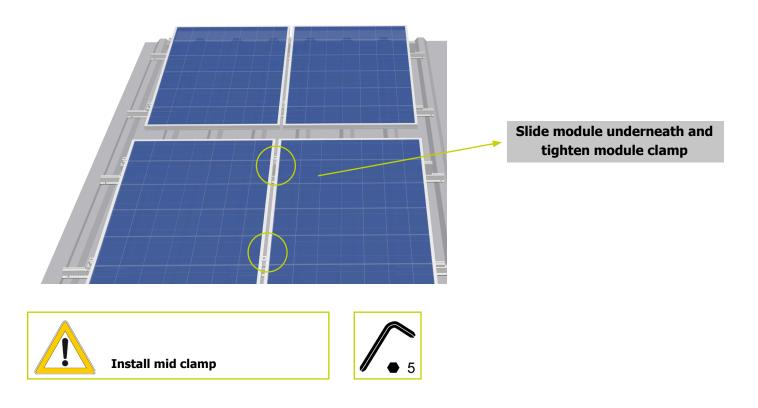
Ensure that the mid clamp clamps both of the module frames at the clamping area defined by the module manufacturer.
