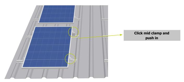
Then slide the next module underneath the module mid clamp, adjust the module clamp to the height of the module's frame and tighten the screw (tightening torque 8-10 Nm).
