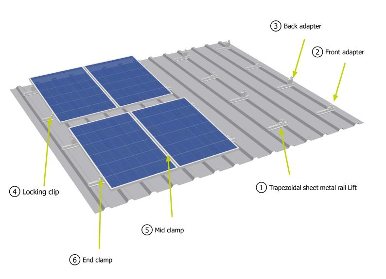
Note: on the following pages, vertical module installation is shown. Horizontal module installation follows the same procedure, but requires clearance to clamp the modules on the short sides.
