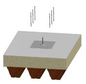
Then place the covering on top and glue it flat to the assembly post and to the roof cladding on all sides.
