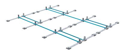
The roll-bars have two functions. Firstly, they raise the static part of the system and facilitate further work like placing the cables and positioning the modules, because the ground rails can no longer move out of place. Secondly, they are used to hold additional ballast.
