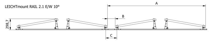
For Area C (connection of the module rows) ground rails in different lengths are available (e.g. for access space or cable laying).
