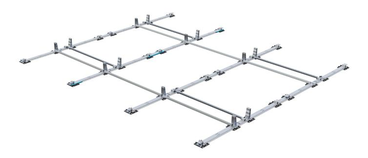
All ground rails have covering cable duct receptacles to protect the string lines from permanent and harmful environmental influences, in particular UV radiation. Installation of the covering cable ducts is possible after every work step of the system installation. The covering cable duct is installed after the cable routing.
