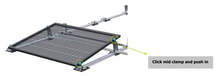
Now push the next module under the mid clamp, adjust the mid clamp to the height of the module frame and tighten the screw (torque 8-10 Nm).
