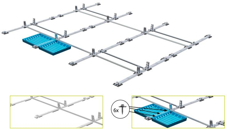
Remove gravel/substrate layer up to the inner edges of the ground rails. The depth of the cleared area over the entire surface should be 50mm from the top edge to guarantee a flat surface for the ballast tray on the remaining layer or roof surface.
