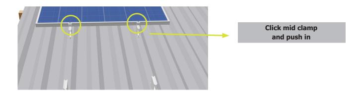
Now slide the next module underneath the mid clamp, adjust the mid clamp to the height of the module's frame and tighten the screws (tightening torque 8-10 Nm).
