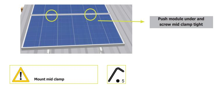
Ensure that the mid clamp clamps both module frames at the clamping area defi ned by the module manufacturer.
