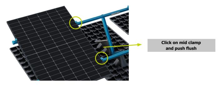
Align the upper row of modules with the aid of a guide or levelling instrument.
