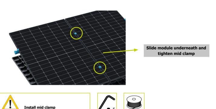
Ensure that the mid clamp grips both of the module frames on the clamping area defined by the module manufacturer.
