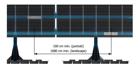
The individual ST profiles are screwed together using the ST connector and 2 M8x20 thread-forming screws each.
