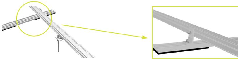
Mount the bracket 40 mm M8 onto the ground rail using a hammerhead bolt M8x25 and a self-locking nut. Ensure that the hammerhead bolt is correctly aligned in the ground rail channel (torque 12-15 Nm).
