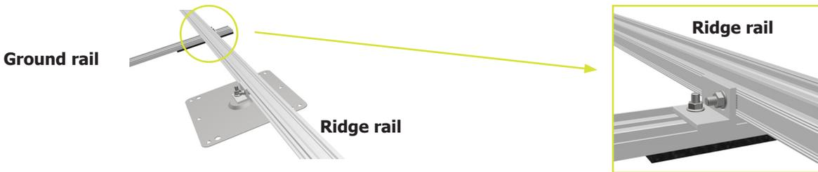
Mount the bracket 60 mm M10 onto the ground rail using a hammerhead bolt M8x25 and a self-locking nut. Ensure that the hammerhead bolt is correctly aligned in the ground rail channel (torque 12-15 Nm).
