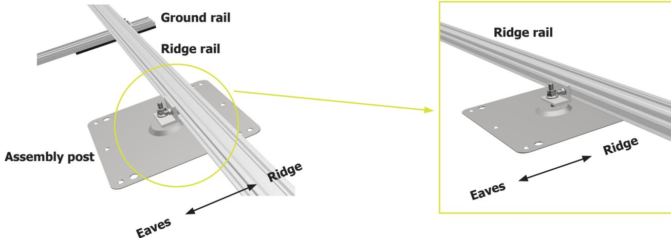
Screw the first M12 locking nut with the flange facing upwards onto the thread of the assembly post and rotate the nut loosely downwards. Place the 60mm M12 bracket with the round hole on the thread. Screw the second M12 locking nut with the flange facing downwards onto the thread of the assembly post and rotate the nut loosely downwards. Repeat the procedure for all assembly posts.
