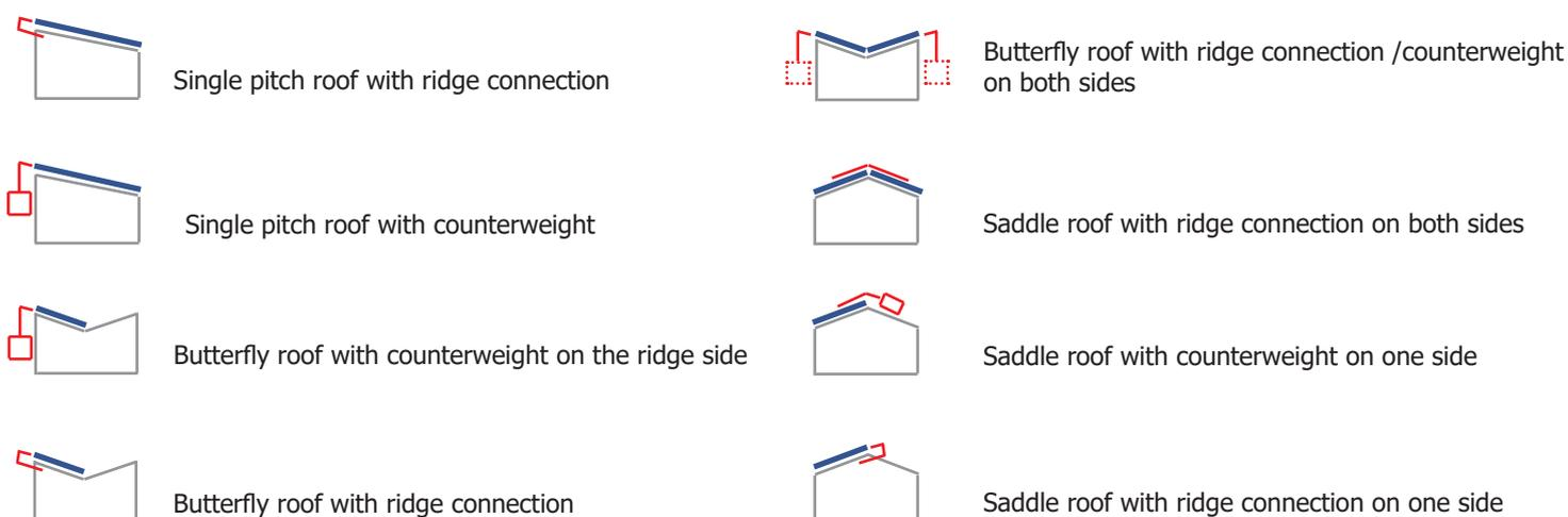
All components are generally made of aluminium and stainless steel. The high degree of corrosion resistance ensures a long service life and offers the possibility of complete recycling.
