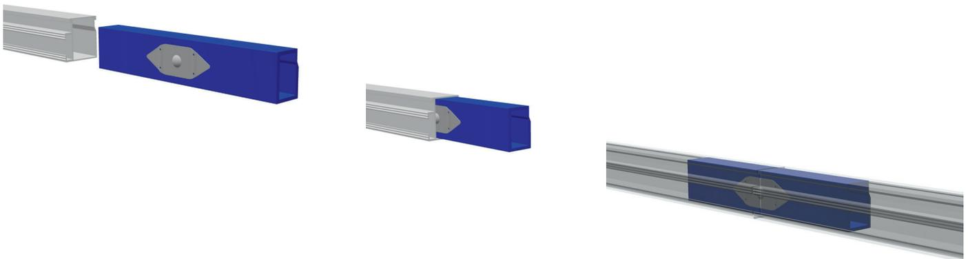
The earthed connection of the mounting rails is established by the splice. Additional earthing of the modules can be achieved via the grounding plate by mounting it under the mid clamps. Before earthing the module, the corresponding specifications issued by the module manufacturer must be observed.
