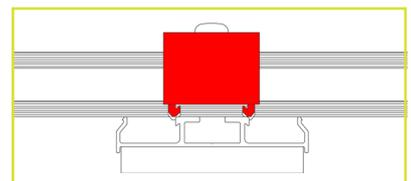
2.3.2 Rail ST-AK 7/47 using bracket 40 mm M8 (for sandwich roofs)
