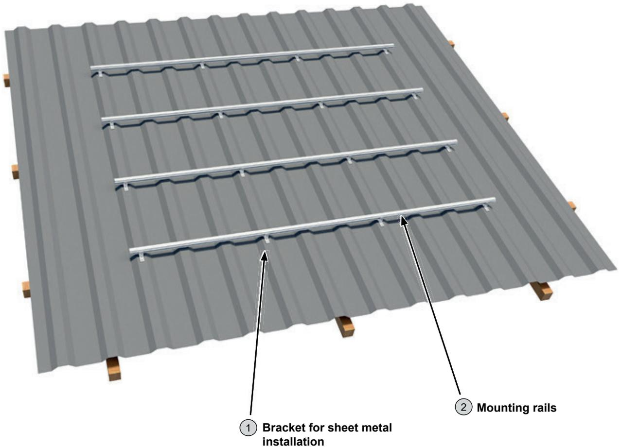
① Bracket for sheet metal installation
