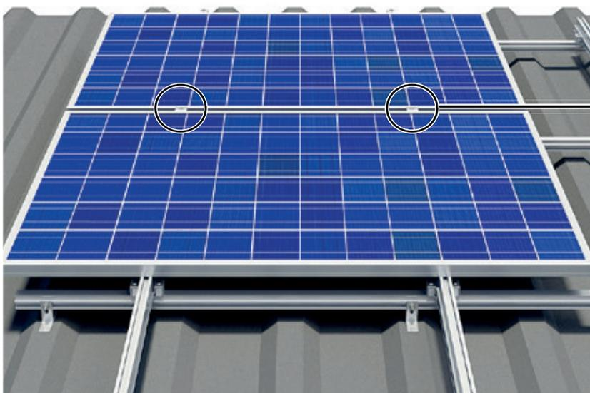
Push module under and screw mid clamp tight
