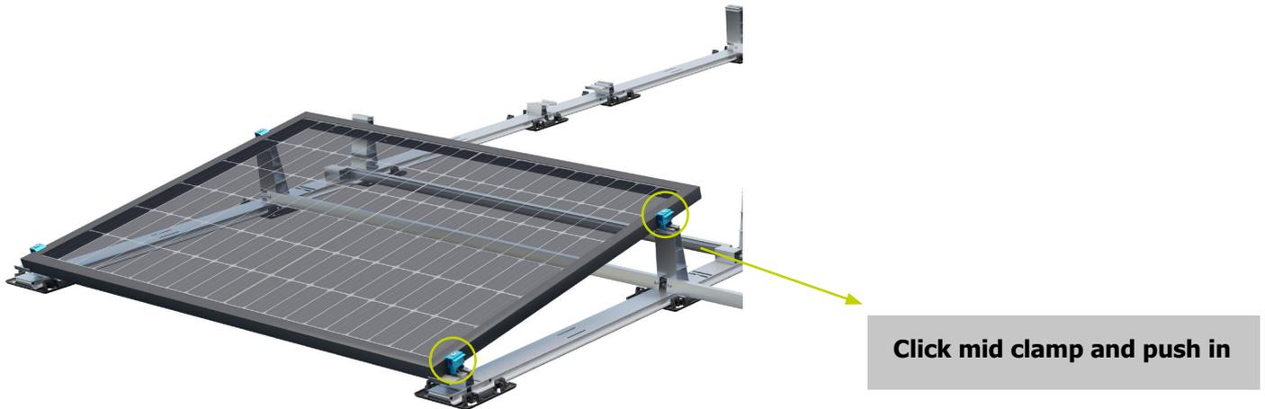
Now push the next module under the mid clamp, adjust the mid clamp to the height of the module frame and tighten the screw (torque 8-10 Nm).
