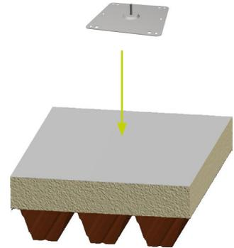
Position the assembly post and screw it into the roof substructure with the appropriate screws OMG HD. The screw connection is established in the raised corrugations of the trapezoidal substructure.
