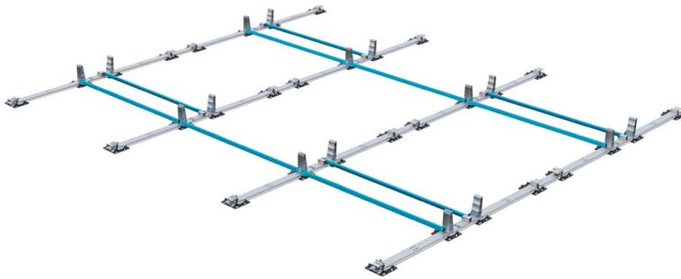
The roll-bars have two functions. Firstly, they raise the static part of the system and facilitate further work like placing the cables and positioning the modules, because the ground rails can no longer move out of place. Secondly, they are used to hold additional ballast.
