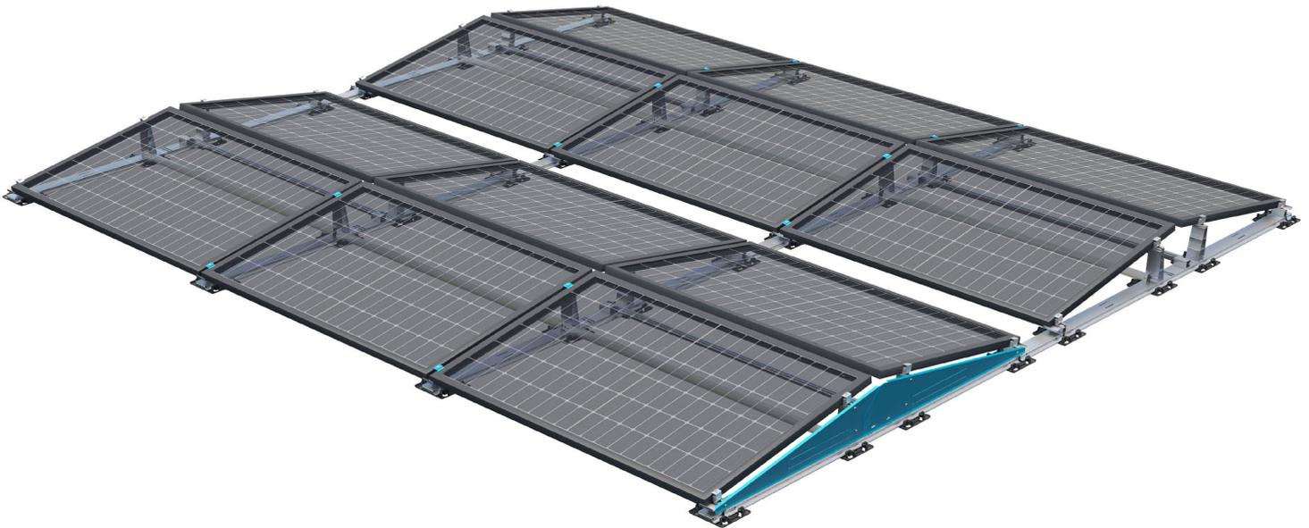
Constructing the system with the side panels improves the cp value, which has a positive impact on the required location ballast, and can also lead to a reduced additional load.
