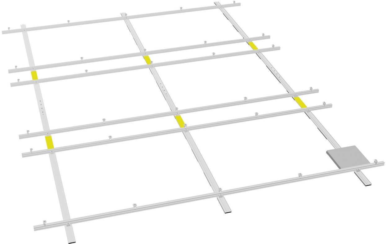
All ground rails have covering cable duct receptacles to protect the string lines from permanent and harmful environmental influences, in particular UV radiation. Installation of the covering cable ducts is possible after every work step of the system installation. The covering cable duct is installed after the cable routing.
