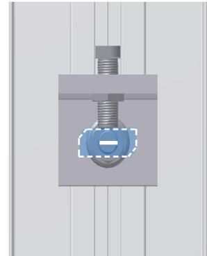
Attach the mounting rail to the bracket using a hammerhead bolt M8x25 and a self-locking nut. Ensure that the hammerhead bolts are correctly aligned in the mounting rail channel (torque 12-15 Nm) and that the mounting rails are installed stress-free. To do this, use the adjustability that is created by the corrugation of the components and the elongated hole.
