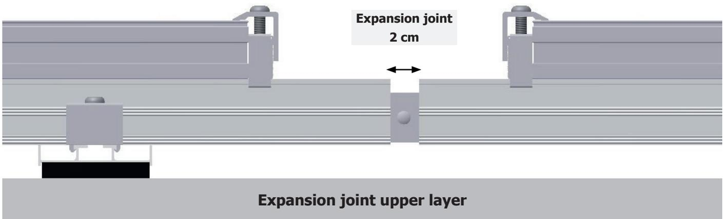
Completed installation of the upper rail layer
