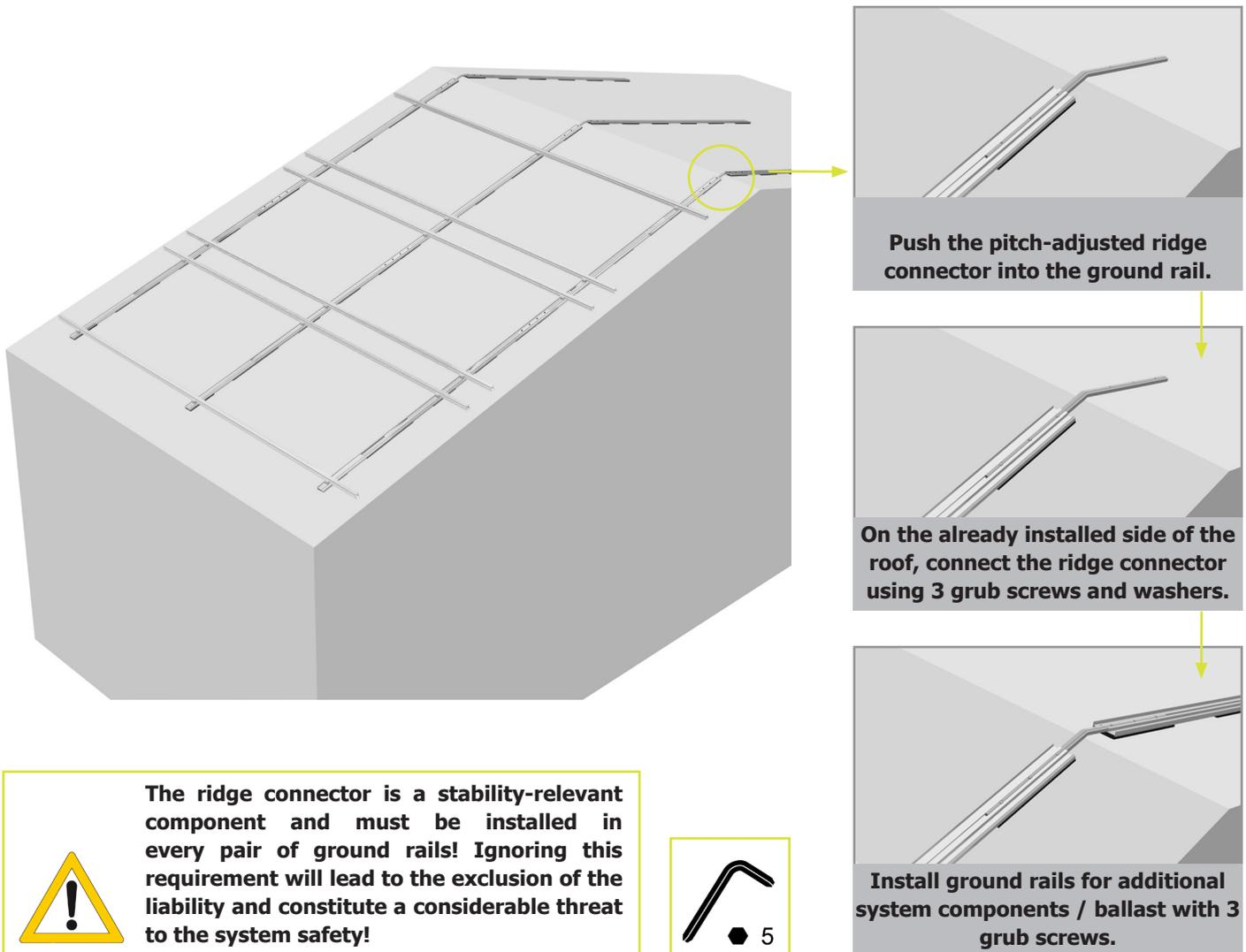
The roof ridge line is to be checked for an even consistent course. Contact of the ridge connector with the roofing must be avoided. If necessary, additional protective mats are to be added.
