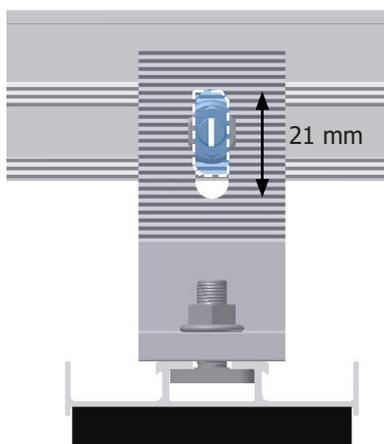
Alignment of hammerhead bolt
