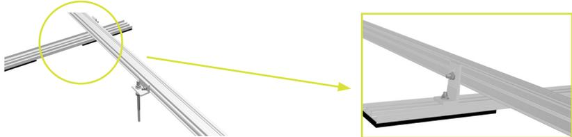
Mount the bracket 40 mm M8 onto the ground rail using a hammerhead bolt M8x25 and a self-locking nut. Ensure that the hammerhead bolt is correctly aligned in the ground rail channel (torque 12-15 Nm).
