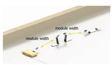
Place the front parts and connectors at approximately the required horizontal distance (module length). The exact distance is adjusted during installation of the module.
