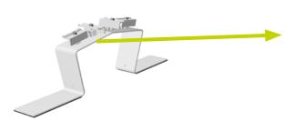
Example of the correct pre-assembly of the individual clamps on the bottom part.
