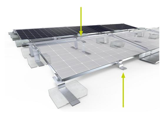
The alpine support at the bottom is only used at the beginning and end of a module field. It is placed in the middle of the module by means of an end clamp and and screwed tightly.
