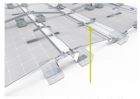
In the middle of a module field, the double support at the bottom is used. It is placed in the middle of the module by means of an end clamp and screwed tightly.
