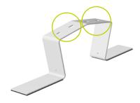
Punching for fixing the clamps at the top of the bottom part.
