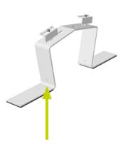
The grounding cable is attached via the round hole in the Top part.
