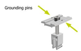
The functional capability of the earthing arrangements for the system via the module mid clamps with grounding pins, and of the system itself, was verified during UL 2703 certification.
