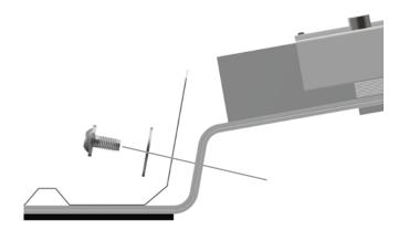
Place a building screen mat (PES, included in the scope of supply) on the left and right side underneath the ballast tray.
