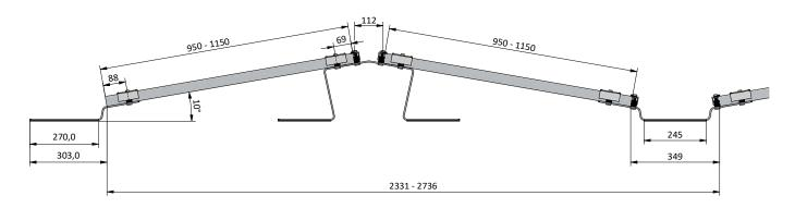
E/W 10° internal shading angle short bottom support
