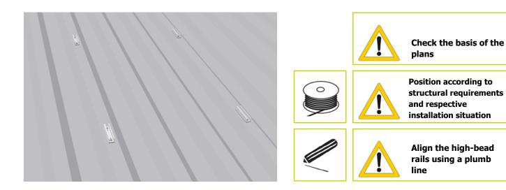
Attach the high-bead rail with the sheet metal screws. Use 2 sheet metal screws per high-bead rail. To prevent water from penetrating between the high-bead rail and the roofing, the high-bead rail must always be mounted on a raised corrugation. The base of the high-bead rail is covered with EPDM sealing strips.
