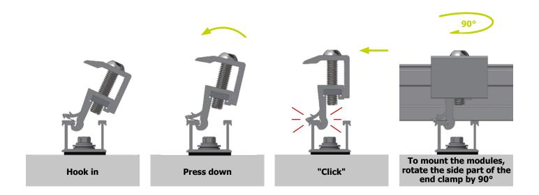
Ensure that the end clamp clamps the module frame at the clamping area defined by the module manufacturer.
