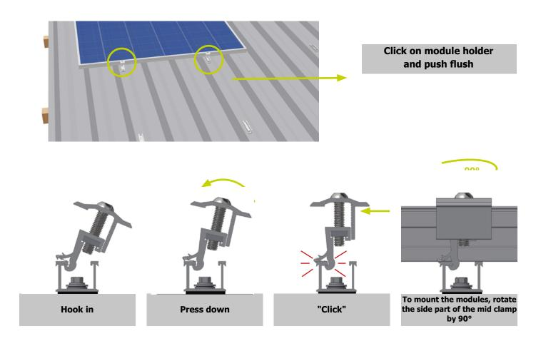
Now slide the next module underneath the mid clamp, adjust the mid clamp to the height of the module's frame and tighten the screws (tightening torque 8–10 Nm).
