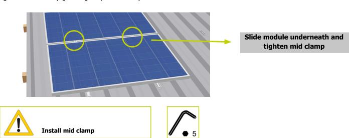
Ensure that the mid clamp clamps both of the module frames on the clamping area defined by the module manufacturer.
