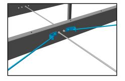
Now fasten the 2 inclined stiffeners/ threaded rods with a length of threaded rods with a length of 2,700mm to the cross member using hexagon bolts M12x30. Two fastening plates are required per threaded rod. Use two washers and two M12 washers and two M12 nuts per fastening plate. In the the corresponding screw caps can be can then be fitted.
