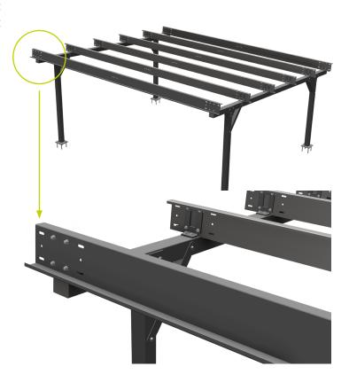
The cross beams of the Carport Double extension are turned by 180° and pushed into the preceding Z-profile in such a way that the perforations overlap.
