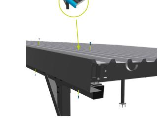
Then the remaining panels are attached to the ridge, overlapping and alternating, using 5.5x19 self-tapping screws on the cross beams from above and below.
