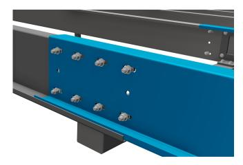
Finally, mount the cross beams to the angles of the last post unit using four M12x35 hexagon bolts, eight washers and four M12 nuts. The screw caps can then be attached.
