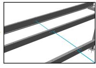
Attach the 5 stiffeners/threaded rods of different lengths (see parts list), staggered one after the other, to the cross member using two washers and two M12 nuts on each side. This means that 4 nuts and 8 washers are needed per threaded rod. Starting from the eaves side, the threaded rods are installed in ascending order of length.
