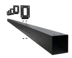
Attach two outer brackets (reversed to the others) to the rafter. Two M12x35 cylinder head screws, four washers and two M12 nuts are needed per angle. The screws are inserted from below.
