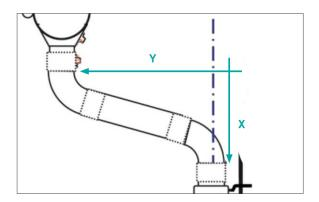
The 3m long downpipe is divided into two elements, downpipe and intermediate piece.
